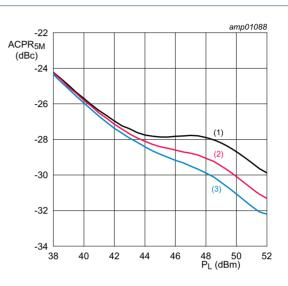
$V_{DS} = 30 \text{ V}; I_{Dq} = 370 \text{ mA}; V_{GS(amp)peak} = 0.85 \text{ V}.$
