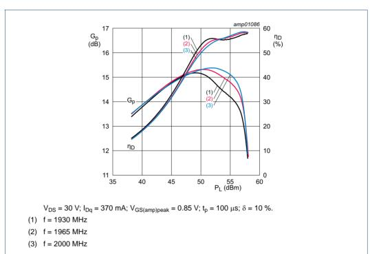
Fig 3. Power gain and drain efficiency as function of output power; typical values
