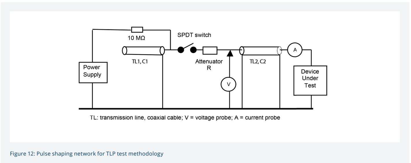
Figure 12: Pulse shaping network for TLP test methodology
