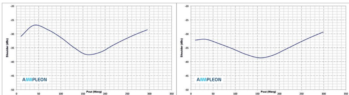
Figure 24: The BLF188XR (right) is extremely suited to linear applications. On the left an older LDMOS generation showing lower linearity at lower power levels, which can be more difficult to pre-correct
