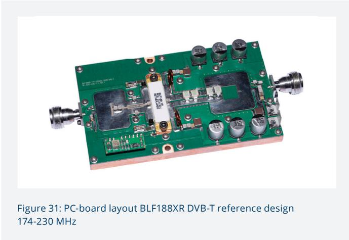
Figure 31: PC-board layout BLF188XR DVB-T reference design
