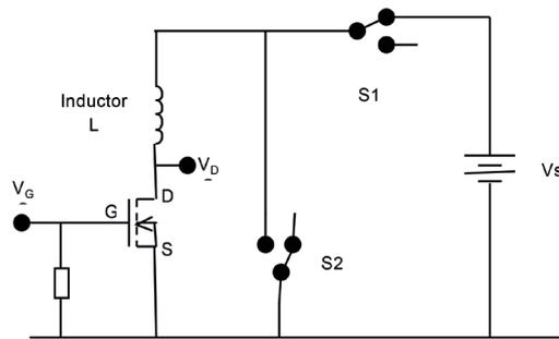
Figure 16: Schematic representation of the Unclamped Inductive Switching (UIS) test setup
