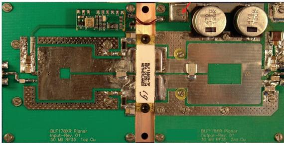
Figure 27: All planar reference design with the BLF188XR for 81.36 MHz
