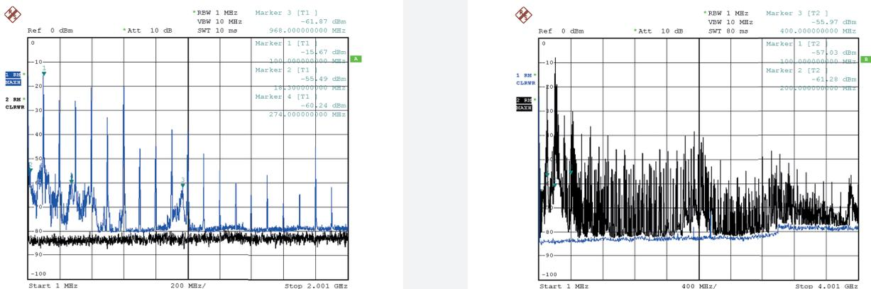
Figure 14: Spectral plot of the BLF188XR (left) and a competitor LDMOS transistor (right) under severe mismatch conditions
