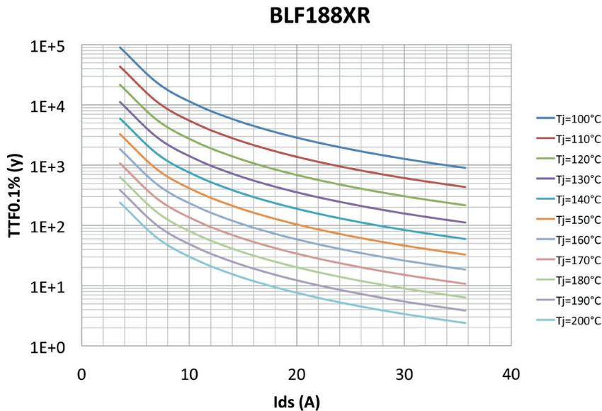
Figure 7: BLF188XR TTF curves for 0.1% failure fraction as function of DC current and temperature
