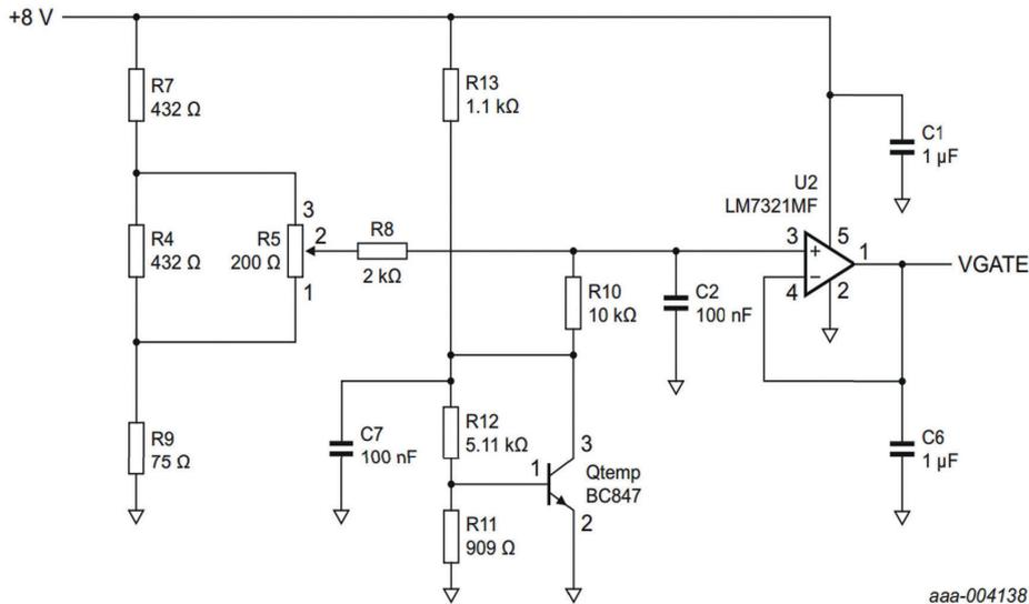
Figure 22: Low  $Z_{SOURCE}$  gate bias circuit
