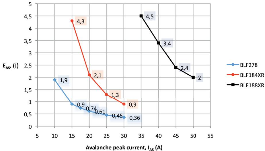
Figure 19: Avalanche test results for the BLF278, BLF184XR and BLF188XR for a single transistor section
