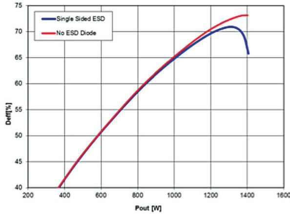
Figure 21: Degradation of drain efficiency as a result of a VBIAS shift when the single sided ESD diode is present. When there is no ESD diode present, a  $V_{BIAS}$  shift will not occur (no rectification)
