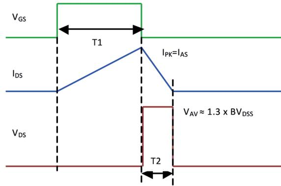
**Figure 17: Timing diagram of avalanche breakdown test**
