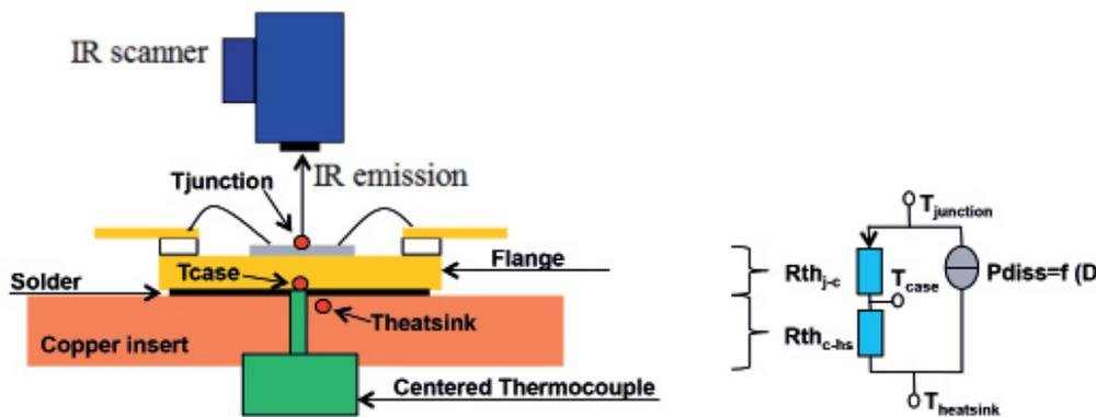
Figure 4: Typical infrared measurement setup
