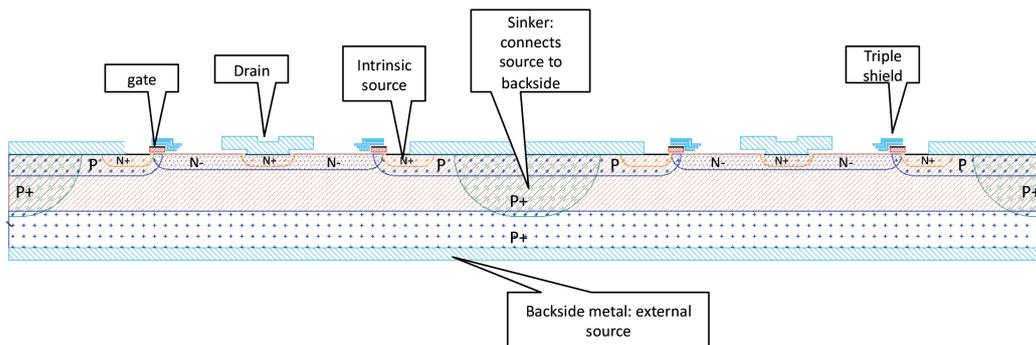
Figure 2: Schematic cross-section of a state-of-the art LDMOS transistor.
