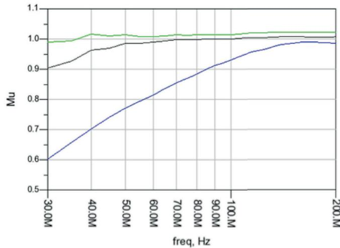
Figure 13: Stability ( $M\mu$ -factor) for the BLF188XR (green line), a competitor LDMOS device (black line), and the BLF278 VDMOS transistor (blue line)
