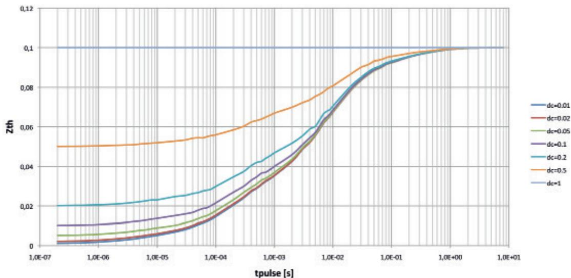
Figure 6: Thermal impedance ( $Z_{th}$ ) for the BLF188XR as a function of pulse width and duty cycle
