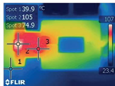
Figure 29: Thermal image of the output transformer of the BLF188XR FM design at 1200 W continuous wave output power
