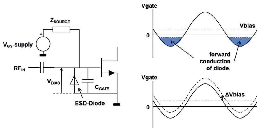
Figure 20: Single-sided ESD diode can cause shift in  $V_{BIAS}$
