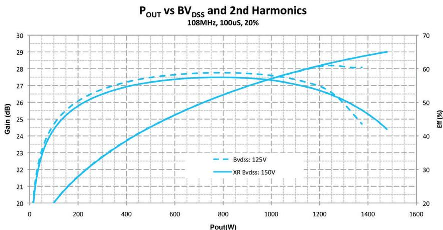
Figure 8: A higher  $BV_{DSS}$  in the case of a high harmonic content improves the output power and efficiency when the device starts to compress
