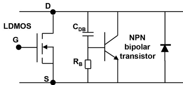
Figure 9: Electrical representation of the LDMOS and the inherently present parasitic bipolar transistor and drain-substrate diode
