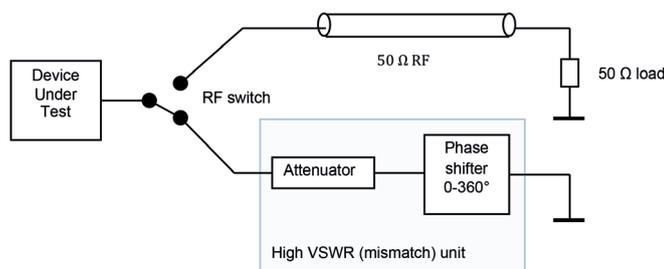
Figure 15: Block diagram ruggedness testing with mismatch unit
