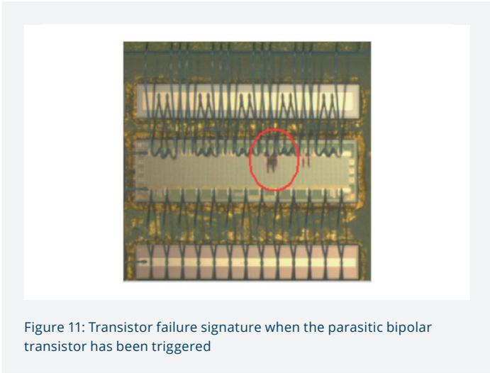
Figure 11: Transistor failure signature when the parasitic bipolar transistor has been triggered
