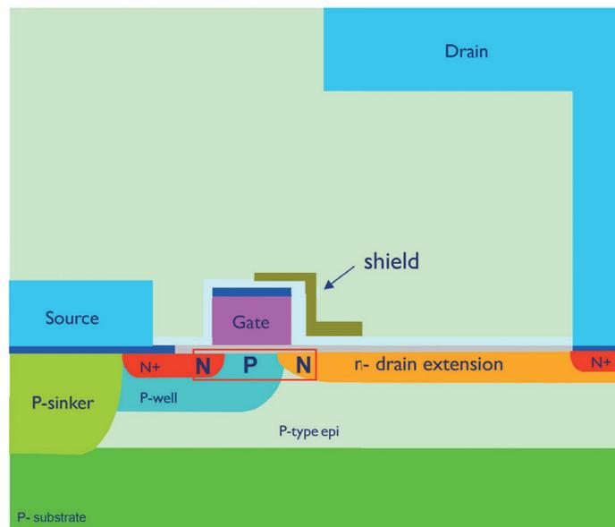
Figure 10: Parasitic bipolar NPN transistor highlighted in the LDMOS structure
