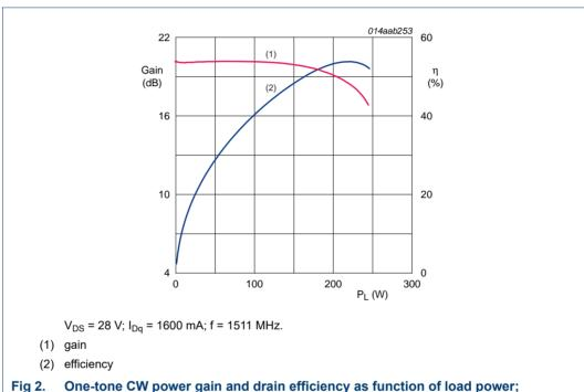
Fig 2. One-tone CW power gain and drain efficiency as function of load power; typical values
