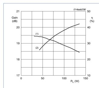
$V_{DS}$  = 28 V;  $I_{Dq}$  = 1600 mA; f = 1511 MHz; carrier spacing 5 MHz.
