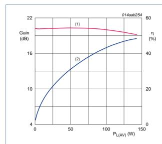
$V_{DS}$  = 28 V;  $I_{Dq}$  = 1600 mA; f = 1511 MHz; tone spacing 0.1 MHz.
