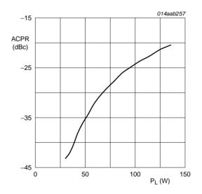
$V_{DS}$  = 28 V;  $I_{Dq}$  = 1600 mA; f = 1511 MHz; carrier spacing 5 MHz.
