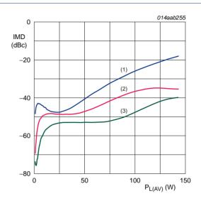
$V_{DS}$  = 28 V;  $I_{Dq}$  = 1600 mA; f = 1511 MHz; tone spacing 0.1 MHz.
