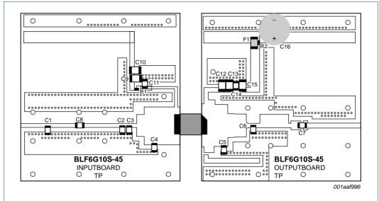
The striplines are on a double copper-clad Taconic RF35 Printed-Circuit Board (PCB) with  $\epsilon_{\text{r}}$  = 3.5 and thickness = 0.76 mm.
