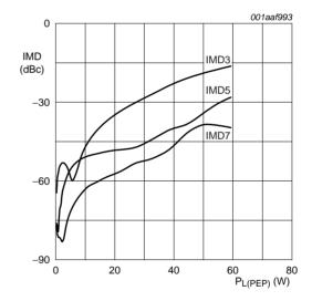
$V_{DS}$  = 28 V;  $I_{Dq}$  = 350 mA;  $f_1$  = 960 MHz;  $f_2$  = 960.1 MHz.
