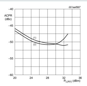
$V_{DS}$  = 28 V;  $I_{Dq}$  = 350 mA; carrier spacing 5 MHz.
