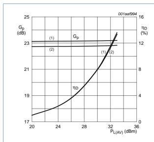
$V_{DS}$  = 28 V;  $I_{Dq}$  = 350 mA;  $f_1$  = 952.5 MHz;  $f_2$  = 957.5 MHz; carrier spacing 5 MHz.
