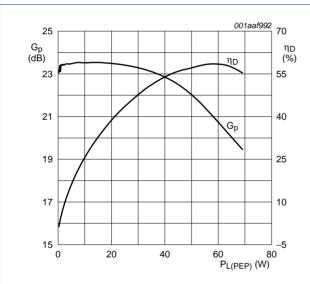
$V_{DS}$  = 28 V;  $I_{Dq}$  = 350 mA;  $f_1$  = 960 MHz;  $f_2$  = 960.1 MHz.
