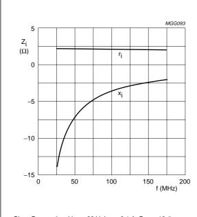
Class-B operation; V\_DS = 28 V; I\_DQ = 0.1 A; R\_GS = 12  $\Omega$ ; P\_L = 80 W; T\_h = 25 °C; R<sub>th mb-h</sub> = 0.2 K/W.
