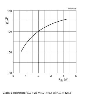
Class-B operation; V<sub>DS</sub> = 28 V; I<sub>DQ</sub> = 0.1 A; R<sub>GS</sub> = 12  $\Omega$ ; f = 108 MHz; T<sub>h</sub> = 25 °C; R<sub>th mb-h</sub> = 0.2 K/W.
