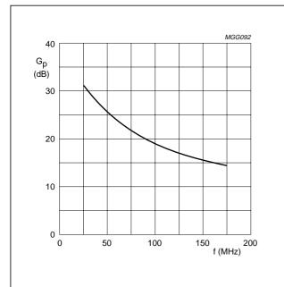
Class-B operation; V<sub>DS</sub> = 28 V; I<sub>DQ</sub> = 0.1 A; R<sub>GS</sub> = 12  $\Omega$ ; P<sub>L</sub> = 80 W; T<sub>h</sub> = 25 °C; R<sub>th mb-h</sub> = 0.2 K/W.
