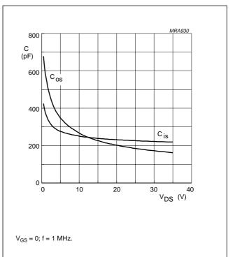
Fig.7 Input and output capacitance as functions of drain-source voltage; typical values.
