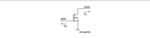
Fig 1. Definition of transistor impedance
