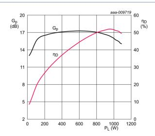
$V_{DS}$  = 50 V;  $I_{Dq}$  = 200 mA; f = 1030 MHz;  $t_p$  = 50  $\mu s$ ;
