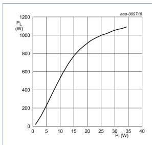
$V_{DS}$  = 50 V;  $I_{Dq}$  = 200 mA; f = 1030 MHz;  $t_p$  = 50  $\mu s$ ;
