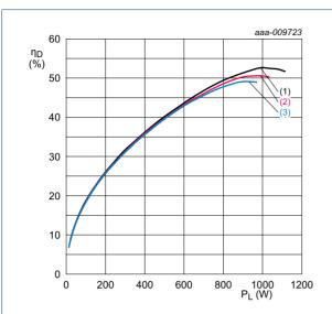
$V_{DS}$  = 50 V;  $I_{Dq}$  = 200 mA; f = 1030 MHz;  $t_p$  = 50  $\mu s;$   $\delta$  = 2 %.
