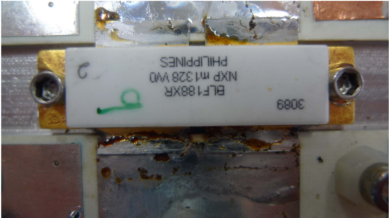
Fig 20. Transistor and 1 mm gap cavities. The drain is at the lower side of the image
